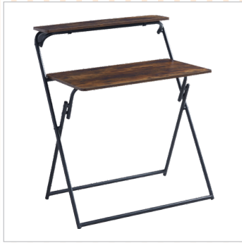
FT001 Size: 31×18×29/37" 1、 Particle board, thickness is 15mm 2、 Tube dia 15mm Thickness 0.8mm 3、 Easy folding
